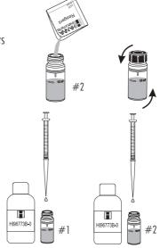
• Add 0.5 mL of HI96773B-0 Oxygen Scavengers Reagent B to each cuvette using the 1 mL syringe.
