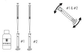
Add 0.5 mL of HI93738D-0 Chlorine Dioxide Reagent to each cylinder (#1 & #2), using a
