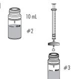
• Filter 10 mL of sample through a filter with a  $0.45 \,\mu m$  membrane into the third cuvette (#3), up to the 10 mL mark and replace the cap. This is the true color.
