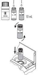
Press the Zero key. The display will show "-0.0-" when the meter is zeroed and ready for measurement.
