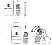
Add 3 drops of HI93703-51 Dispersing Agent to each cuvette, replace the caps and invert gently to mix for about 30 seconds.
