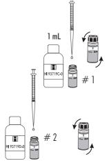
Add 1 drop of HI93719D-0 Magnesium Hardness Reagent D to the second cuvette (#2), replace the cap and invert the cuvette several times to mix. This is the sample.
