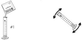
Add 0.5 mL of H193738C-0 Chlorine Dioxide Reagent C to each cylinder (#1 & #2), using a 1 mL syringe, cap, and invert several times to mix.
