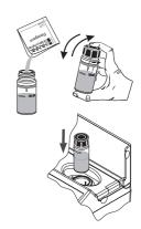
• Reinsert the cuvette into the instrument and close the lid.
