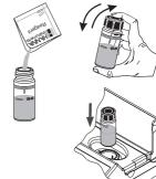
Press Timer and the display will show the countdown prior to the measurement or, alternatively, wait for 2 minutes and press Read. When the timer ends the meter will perform the reading. The instrument displays the result in mg/L ozone (0<sub>2</sub>) (chlorine free sample only).
