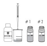
• Add 1 drop of HI93720C-0 Calcium Hardness Reagent C to one cuvette (#1).
