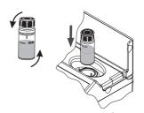
Press the Zero key. The display will show "-0.0-" when the meter is zeroed and ready for measurement.
