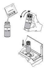
Reinsert the cuvette into the instrument and close the lid.
