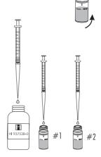
• Add 0.5 mL of HI93753B-O Chloride Reagent B to each cuvette using the second 1 mL syringe.
