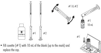
Press the Zero key. The display will show "-0.0-" when the meter is zeroed and ready for measurement.
