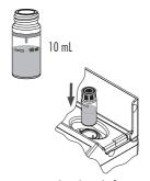
Press the Zero key. The display will show "-0.0-" when the meter is zeroed and ready for measurement.
