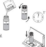
• Reinsert the cuvette into the instrument and close the lid.
