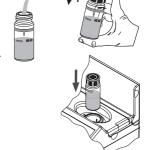
Press Timer and the display will show the countdown prior to the measurement or alternatively, wait for 1 minute and press Read. When the timer ends the meter will perform the reading. The instrument displays the results in mg/L of chlorine (Cl<sub>n</sub>).
