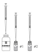
• Replace the caps and mix each cuvette by inverting for approximately 30 seconds.
